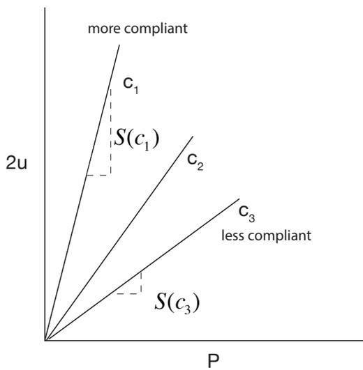
To measure  $\frac{dS}{dc}$  we make DCB (double cantilever beam) specimens with different crack lengths, and measure the compliance with the application of small loads (less than those that may cause fracture) which will give plots such as
