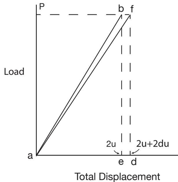
Note: The specimen has unit thickness normal to the plane of the paper. Therefore, the load  $P$  has units of  $\text{Nm}^{-1}$  (not just Newtons)
